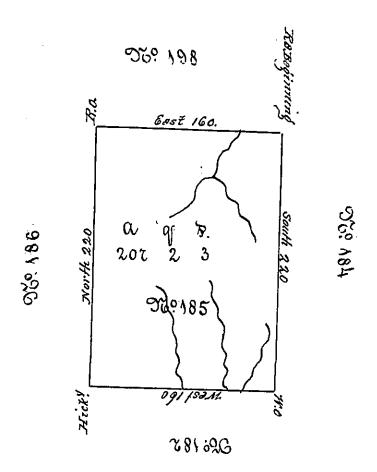
The above is a Draught of a Durvey made the 9th Day of June 1786 In Bursnance of Instructions from the Durveyor General on the Waters of Connegnenasing on the West Side of the Olio two in Destrict 56.2 being point of the land to be sold for the Tederuption of the Depreciation betificates Containing two hundred seven Acres one half and three poles with Asnal allowance of 6 # 0!
